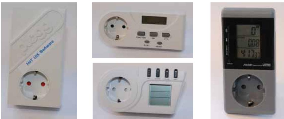
**Figure 3. Selection of different end-user electric power meters, 15 to 60 €/ each. Wireless device on the left, devices with an interface and a display in center and on right.**
