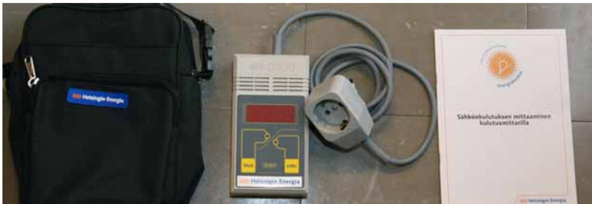
**Figure 3. Meter package including the Christ Elektronik CLM200 power meter. The device has only two operation modes, “Watt” for electric power and “kWh” for consumption.**
